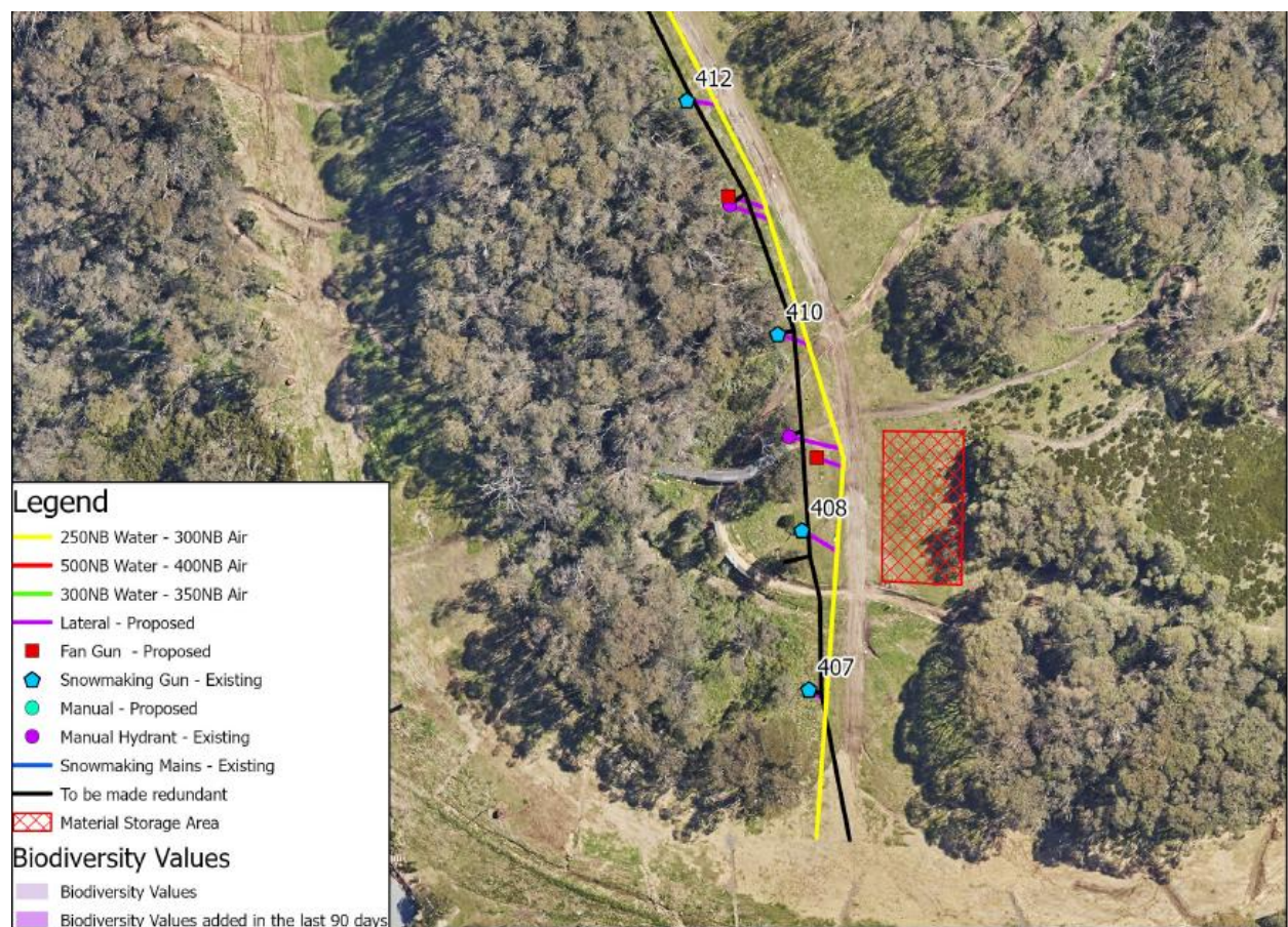
Figure 8 | Works in vicinity of 'Cat Shed', relocated manual hydrant as shown (Source: Applicant's Documentation)
